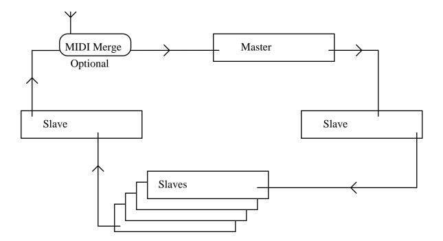
Any DN3600 in the loop can be designated as the Master by entering the Slaves sub menu (press **Utilities, More..., Slaves** on the DN3600). The other DN3601 and DN3600 units in the loop will automatically configure themselves as slaves, with the first being number 1, the second being number 2 and so on. Each slave will display its number on its own front panel LED display. A maximum of 64 units may be connected in this way (65 including the Master).
